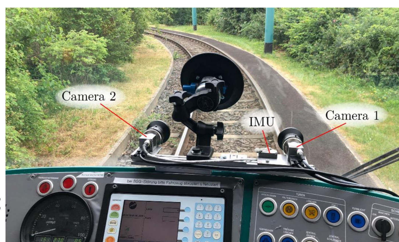
Fig. 2: Sensor consisting of two cameras (stereo) and IMU.
